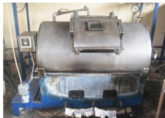
Gambar 3. Alat Penggoreng Vacuum Frying
